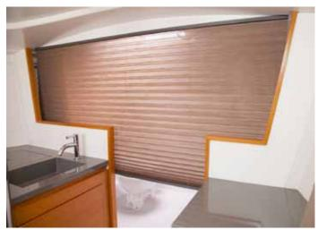
A privacy blind to separate the forward berth or when the heads is in use. Alternative arrangements offer a separate heads compartment
