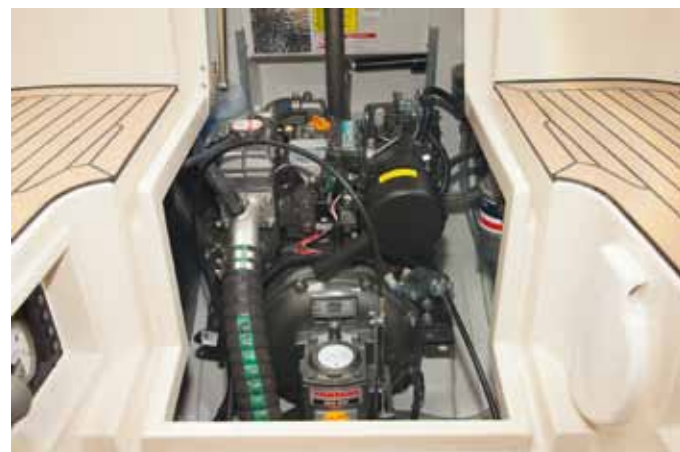
Unusually, the twin-cylinder Yanmar diesel is mounted abaft the cockpit to avoid a raised sole or companionway. Access is good, and from aft too
